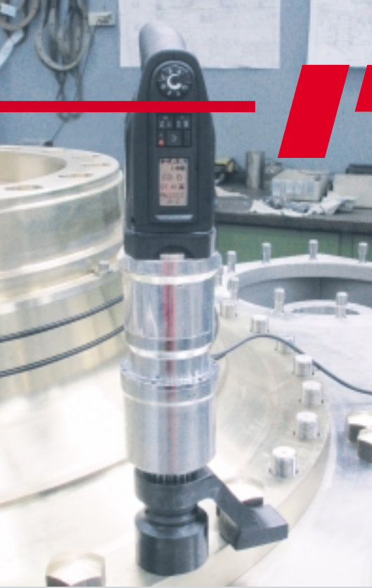
Electric rotation tensioner EDS-250, bolting of rudder propellers
