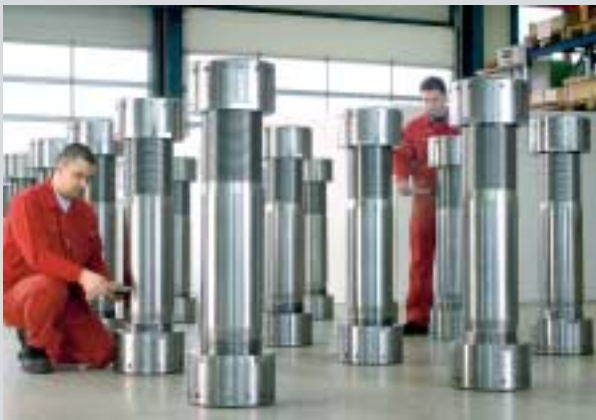
Close-tolerance bolts M 245 for water turbines
